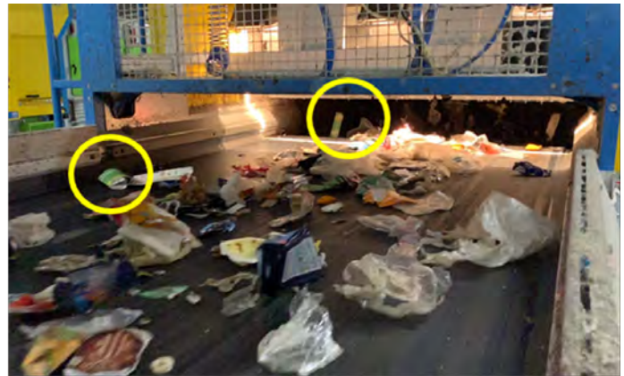
Picture 2: Near Infrared (NIR) Sortation Equipment Showing Paper Can Sortation
