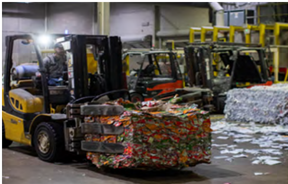
Picture 3: Paper cans on forklift (left) are fed into the pulping process and blended with other recycled paper products (right)
